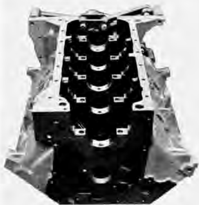
SOHC uses same basic block as 427 wedge. Oil system must be checked, some passages enlarged, others blocked.
