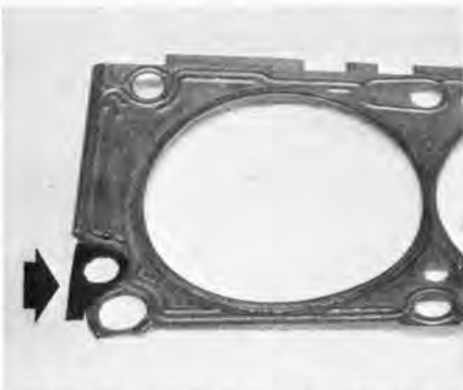
Stock 427 steel shim head gasket is one to use, but small velumoid insert must be used to seal around the drain-back hole.
