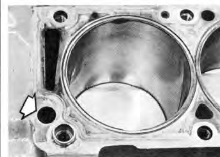
Shot of number 8 cylinder shows O-ring groove, small valve reliefs and rear oil drain-back hole. Note old gasket marks.
