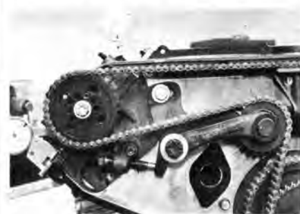
Proper tightening of chain tensioner is vital. Continuously turning engine over during tightening helps eliminate slack.
