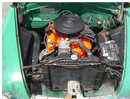
To allow for the wider V-8 the inner fenders were modified.
