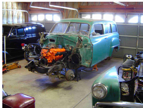
The 318 and Torqueflite is a lighter package than the 6 cylinder and 3 speed it replaced.
