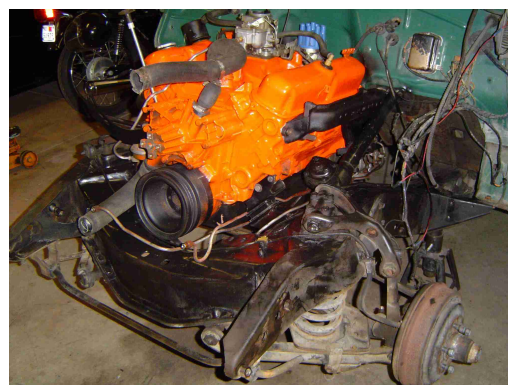
Mounted a little higher than the 6 cyl and 1 1/4" to the left the 318 is a good fit.
