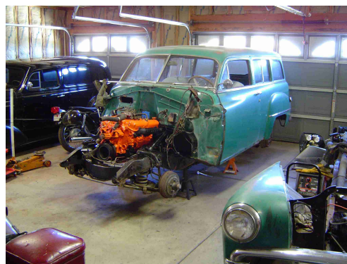
The 318 and Torqueflite is a lighter package than the 6 cylinder and 3 speed it replaced.
