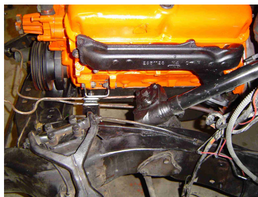
The Duster exhaust manifold tucks behind the stock steering
