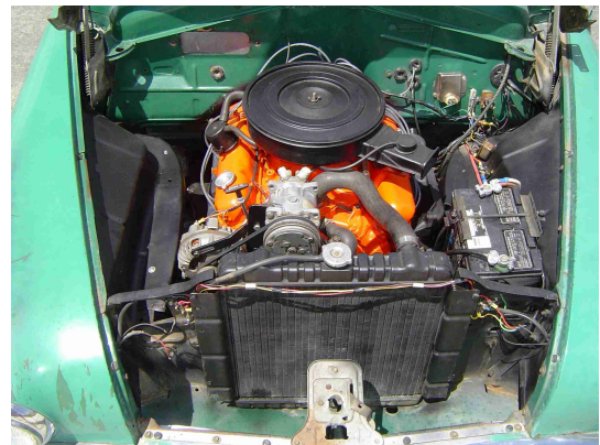
To allow for the wider V-8 the inner fenders were modified.
