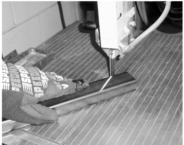
Cutting diagonal brace
