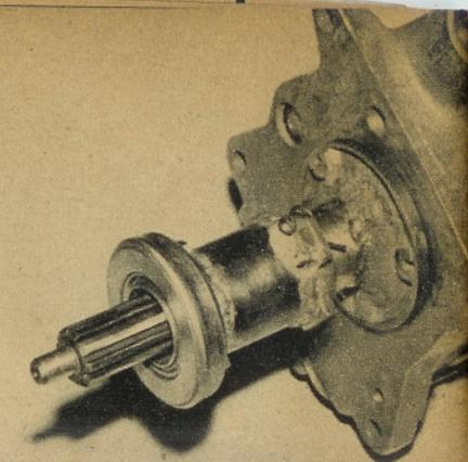
...had to be lengthened  $2\frac{1}{4}$  inches, by welding stock to the original shaft, then re-machining and cutting splines, so the unit would reach the pilot bearing in the Chrysler flywheel. Now the unit is ready to be installed.
