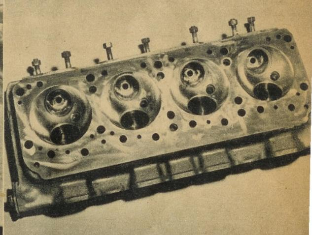
...all passages were polished to a mirror-like finish. Similarly, the combustion chamber surfaces were given the polish treatment. When openings matched gaskets, the heads were placed on engine and torqued down.
