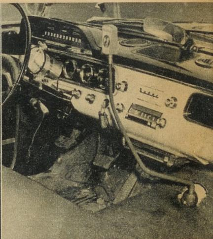
Following present practice, the longest lever possible was used. A hole was cut in the floor to allow protrusion of gear selector housing. Note electric tachometer mounted on steering column where it is easily readable by driver.
