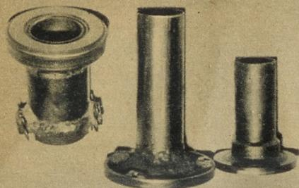
An entirely new front transmission bearing retainer and a throwout collar had to be fabricated. The stock La Salle retainer is shown at the left, with special components in center and at right. The pilot shaft...
