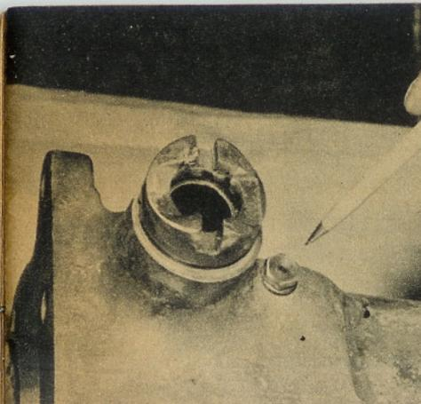
La Salle boxes were never made for continuous running at high speed. The pencil indicates a breather installed to prevent pressure from building up in the box and let foaming gear oil leak through the gear selector opening.
