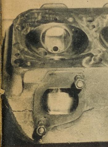
The heads were really given the works—since they're perhaps the most important items in a healthy, power-producing engine. The intake and exhaust ports were enlarged as far as the gaskets would allow, then...
