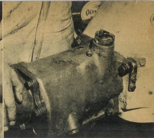
Bellhousing was smaller than face of transmission so a bracket had to be bolted to it so upper right case ear could be bolted down. Note how far forward gear selector is, placing stick up under the dashboard.
