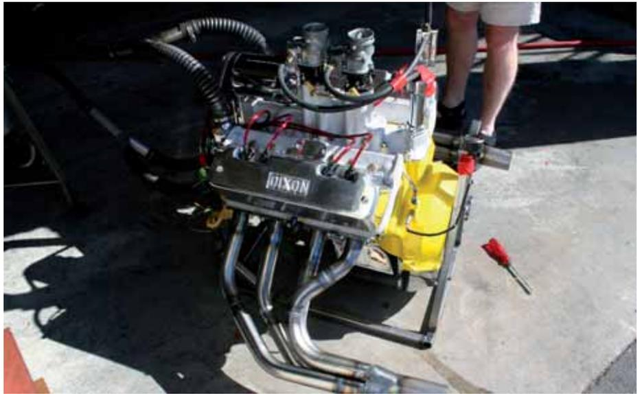
Richards and the Dixon V8 conversion. From there some 'outside the square' thinking led to a concept for a genuine nostalgic traditional hot rod - a Dixon V8 powered '32 roadster. We've been lucky to be riding shotgun on this project and were invited to the initial break-in and dyno tests to prove reliability and establish a tune-up and horsepower levels.
