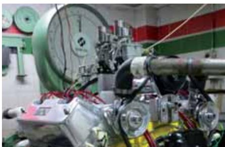
Two Jerry Jobe-built Stromberg 48s with 51 jets were fitted to the rare Tattersfield twin carb intake then the engine warmed up ready for final power pulls.
