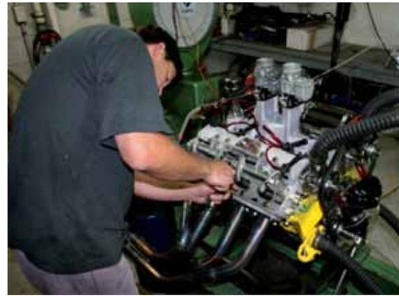
*After a thorough break-in the valve lash was checked; adjusters needed replacing.*
