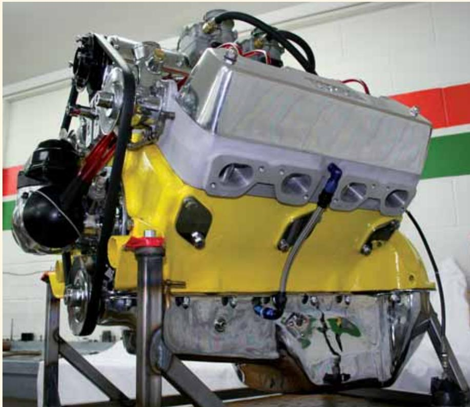
Note the oil return line from the head to the sump. Three stock exhaust ports in the block are blocked off. Exhaust now exits via 4 OHV exhaust ports in the cylinder head, thereby eliminating hot exhaust passing through the block. A major performance weakness in the flathead's design, was overcome by the Dixon conversion.
