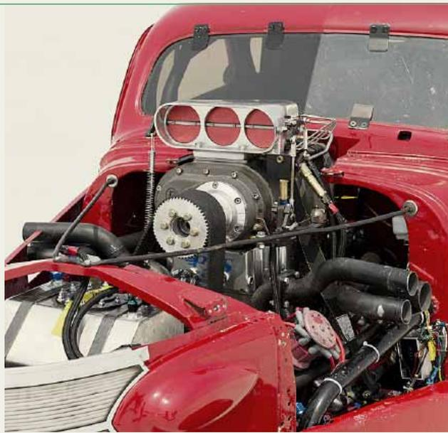
high thermal reserve without requiring air through-flow. The routing of the coolant has been improved by taking it into the lower block and out of the heads. For oiling there is a dry-sump system with priority to the mains and full pressure to the lifters. These lifters ride in blocks that, once again, are tied together to increase strength, rigidity and reliability.
