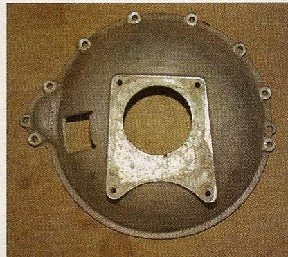
> This is a Cragar adapter for pre-'64 Ford three- and four-speed transmissions. It uses the Ford clutch fork. Note that it doesn't have any provision for mounting a dust shield on the lower portion of the bellhousing, allowing the flywheel and clutch to be exposed to dirt and rainwater. Even so, this unit is nice because you can run a Ford three-speed overdrive behind it, which is a pretty common trans.
