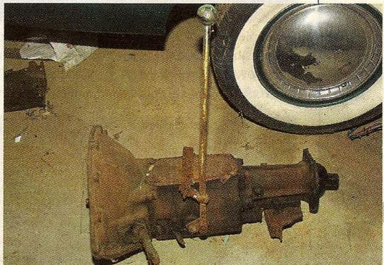
> We picked up this six-Bolt Buick trans a few years ago, complete with a homemade shifter that mimics the DragFast design. The pivot acts as a fulcrum: When the shift handle is pushed toward the passenger side, it pulls the shaft out from the trans to engage First and Reverse. When the shifter handle is pulled toward the driver, the shaft slides into the trans to engage the Second and Third cluster.
