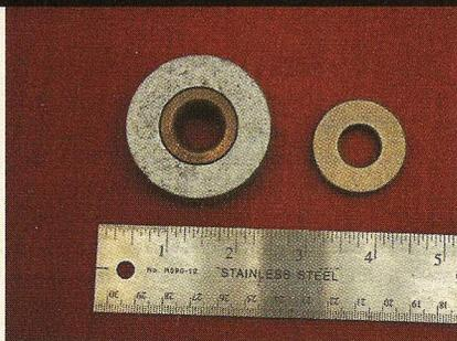
> Our Trans-Dapt bellhousing came with a large-diameter aluminum doughnut with a bronze pilot bushing to convert the Dynaflow crank for use with a manual trans. The bronze bushing on the right is an N.O.S. Oilite bushing for the back of manual cranks, though we found a roller bearing in our '54 Special crank (it eventually failed, killing the input shaft of our five-bolt trans).
