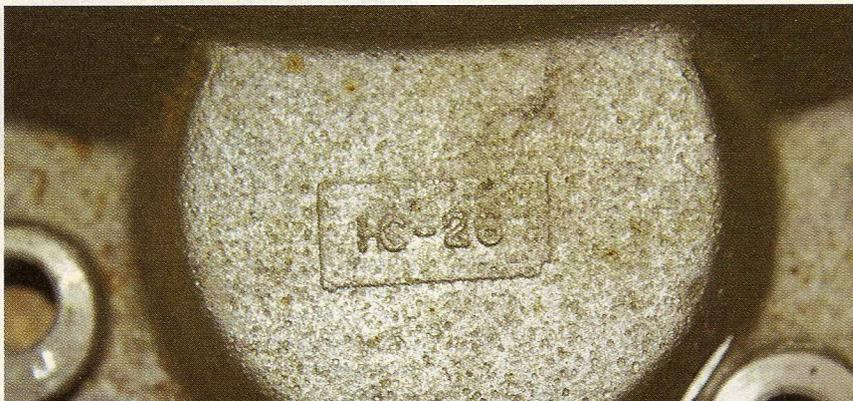
> The ID number for TD bells is typically found on the starter boss and is hard to read even on a perfectly clean example.
