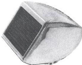
This new streamlined flame arrester cast of aluminum and polished to a chrome like finish. Stainless steel element. Unit is 3-3/4" high, 4-5/8" wide and 5-1/4" long. Element removal quick and easy for dragging.
