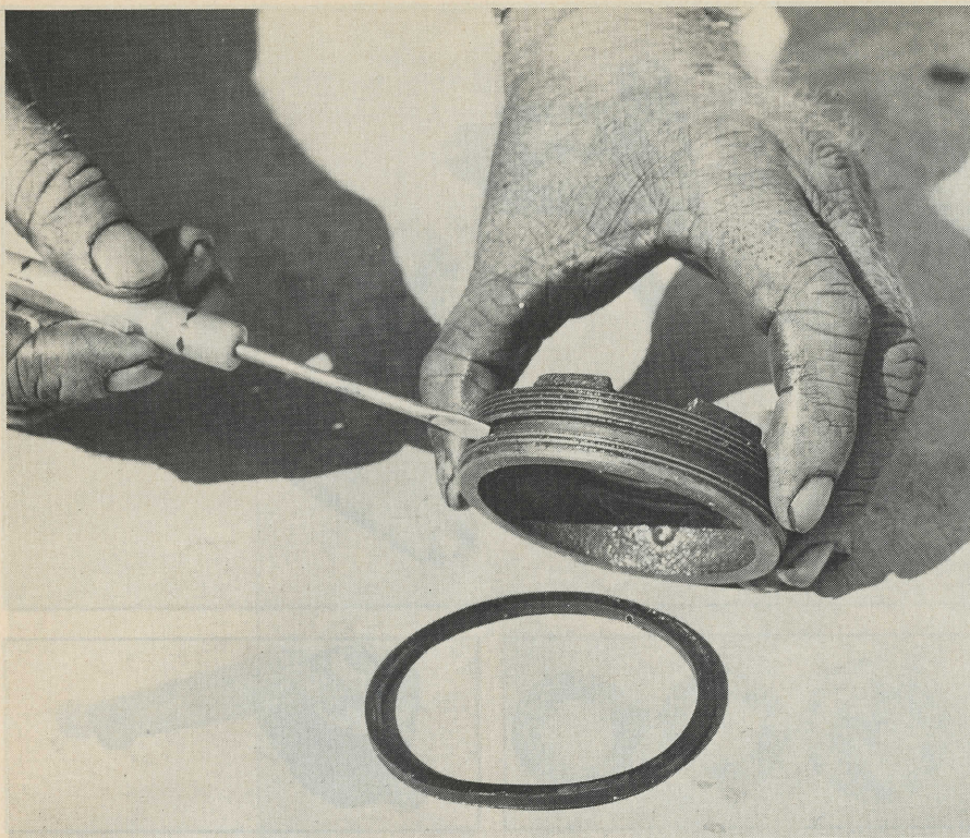
Typical shock for 1941 to '48 Fords. Trouble generally starts around arm/shaft area with fluid leakage.
