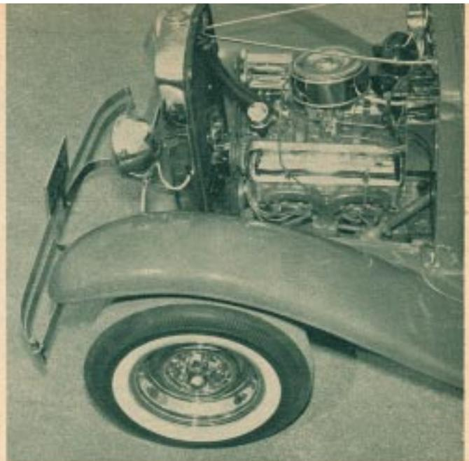
*Sitting between the '31 Chevy frame is a stock '57 Chevy mill. The chroming was slight but tastefully done. The engine is bolted to a '57 Chevy transmission which has a modified floor shift.*
