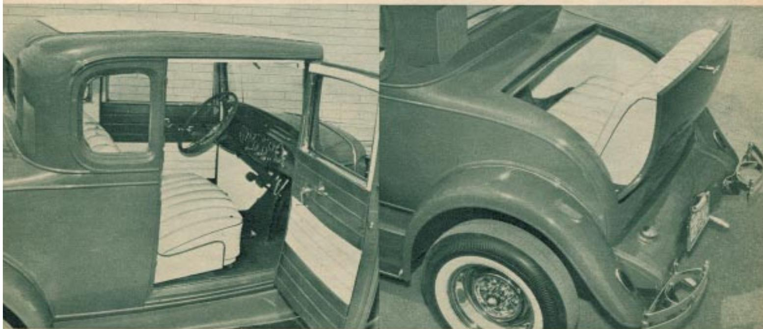
*Sharp looking upholstery was done in red and white Naugahyde by owner. Steering wheel is '58 Chevy Impala and dash gauges are Stewart-Warner. Swing pedals are used and hand brake is stock.*
