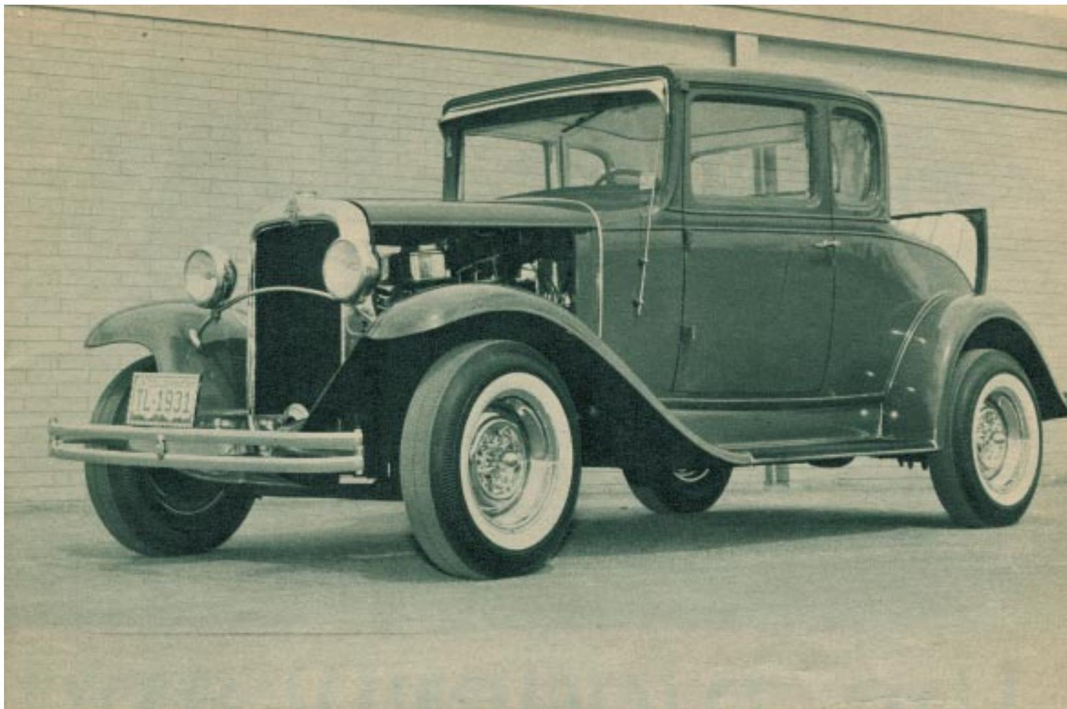
*Brakes on the coupe are '56 Chevy and all the front and rear suspensions are stock '31. The tires up front are 6:70 x 15 and rears are 7:10 x 15 for more traction. The steering is from a '53 Ford pickup and the headlights are seal beams wired to the 12-volt system. Side panels were eliminated to show off the engine compartment and to help keep the engine cool while driving.*
