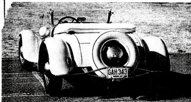
Bracy built and installed the nerfs; workmanship is top. Taillights are stock '38 Ford. Notice the neat top boot.
