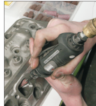
Using a Standard Abrasives deluxe head porting kit from Eastwood Company, we gasket match ported the heads. The intake side required little work, although the center two ports on the exhaust side have some restriction.
